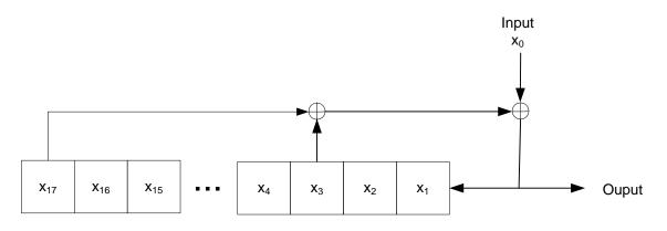
Preload shift register with 0x01prior to start
