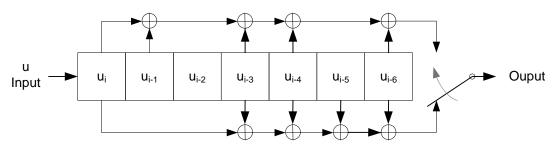
Figure 3-5 Block Diagram of Rate 1/2 k=7 Convolutional Encoder
