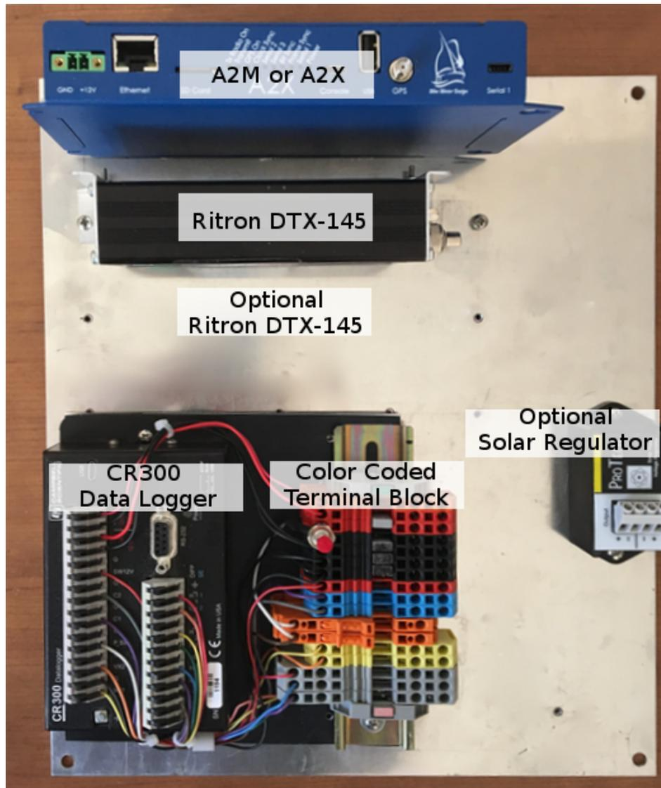
Image showing the layout of Blue Water Design's flexible backplane. Dimensions are 10.88" x 12.75". Cables are not shown for clarity.
